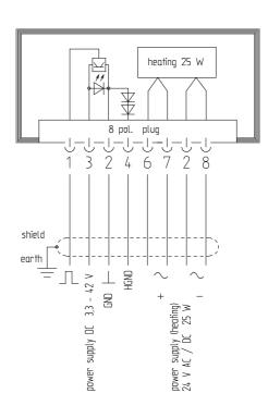
Pole figure of the 8-pole plug connector (DIN 45326) with view on the soldered connection side of the socket insert
