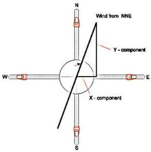
As the speed of sound is very dependent on the air temperature, the propagation time of the sound is measured on both of the measurement paths in **both** directions. In this way, the influence of the temperature dependent speed of sound on the measurement result can be eliminated by subtracting the reciprocals of the measured propagation times.
